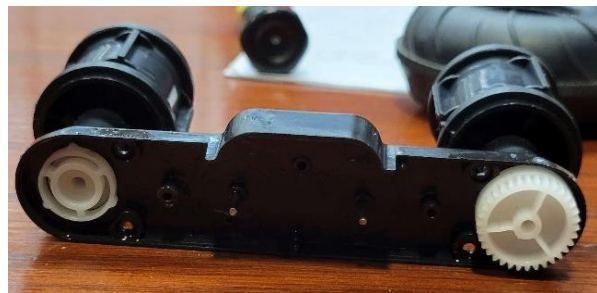
Fig. 8. Back-view of the internals of the wheels. One gear is taken off to show the relationship between the base gears and the wheel gears. (Pak, 2023)
