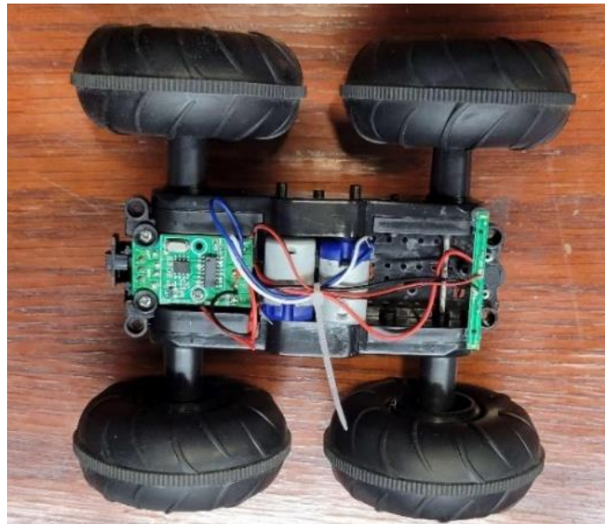
Fig. 3.1. Top view showing the internals of the RC car. (Pak, 2023)
