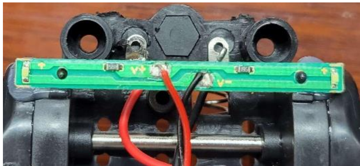
Fig. 5. The circuit board at the front and back of the car, each side contains a white LED. (Pak, 2023)
