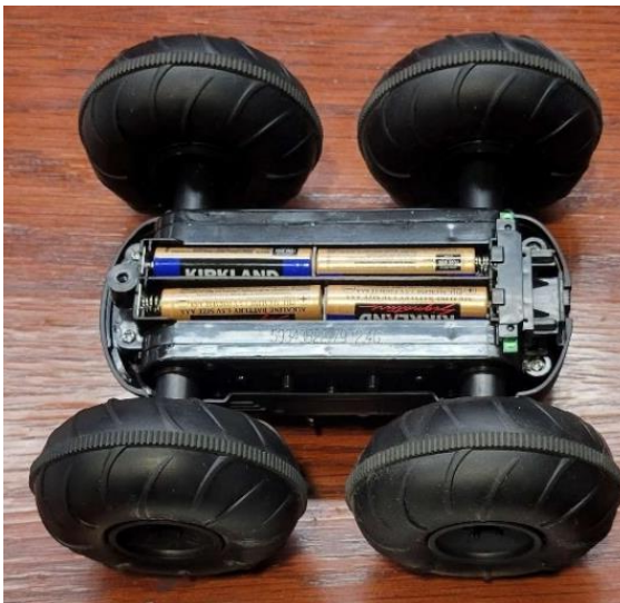
Fig. 3.2. Bottom view showing the battery compartment. (Pak, 2023)
