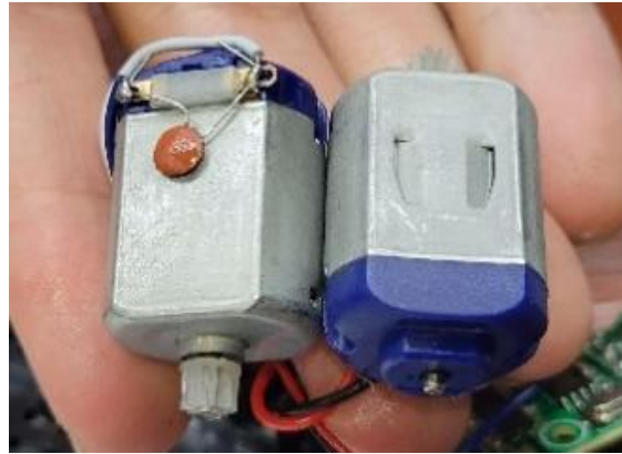
Fig. 6. Motors used to power the rotation of the wheels. Each one has a small gear attached to the shaft. (Pak, 2023)
